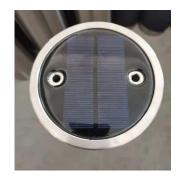
5. After following above steps and making sure the LED Solar Powered Bollard can light up, you can now tighten the screws close the cap.
