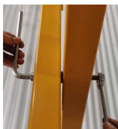
Step 4: Tighten using hex key and spanner
