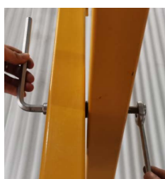
Step 4: Tighten using hex key and spanner
