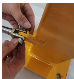
Step 5: Gas strut installation
