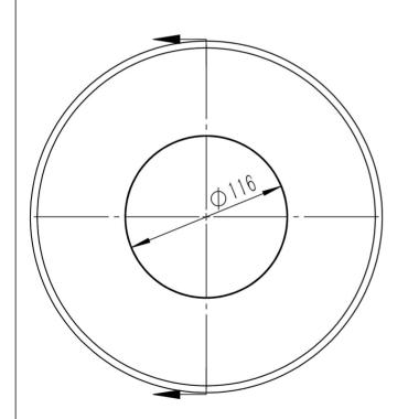
**Base Cover for 114mm Surface Mount Bollard**
